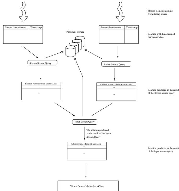
Figure 2: Conceptual data flow in a GSN node
